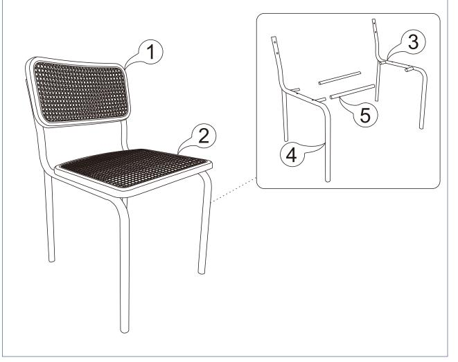
STEP 3: Connect steel frame(3), (4) and connecting tube(5), as the instruction show.
