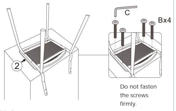
STEP 6: Turn over the steel frame and put it on the floor. Connect the back(1) and steel frame, using bolt B and fasten with Allen Key C, as the instruction shown.
