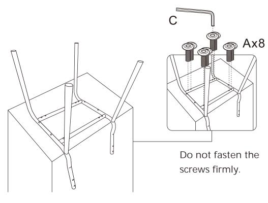
STEP 5: Connect seat(2) and steel frame, using bolt B and fasten with Allen Key C, as the instruction shown.
