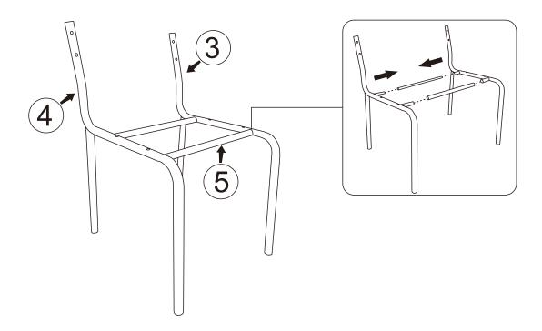
**STEP 4:**Turn over the steel frame and put it on the desk, using bolt A and fasten with Allen Key C, as the instruction shown.
